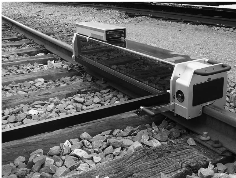
Fig. 7. New mbbmRM1200 rail roughness measurement device on a test track.
